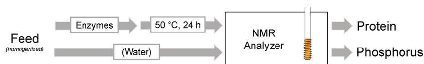
**Fig. 2 – Schematic illustration of procedures proposed for low-field NMR quantification of protein (upper track) and phosphorus (lower track) in livestock feed samples.**
