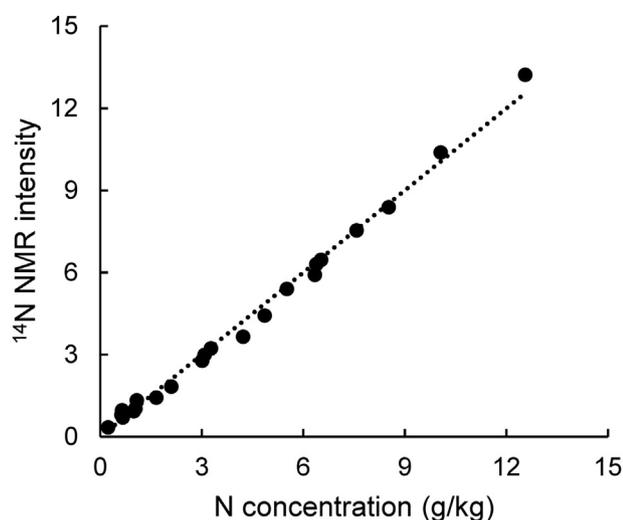
**Fig. 1 – Calibrated  $^{14}\text{N}$  NMR intensity versus calculated nitrogen concentration for 22 aqueous solutions of small molecule compounds. The samples include 18 distinct amino acids, urea, a dipeptide (GlyGly), and two mixtures of amino acids. The  $^{14}\text{N}$  QCPMG signals were recorded at 4.63 MHz using a recycle delay of 30 ms and accumulation over 1 h for each sample. See [supplementary material](#) for a list of included samples and details on NMR experiments.**
