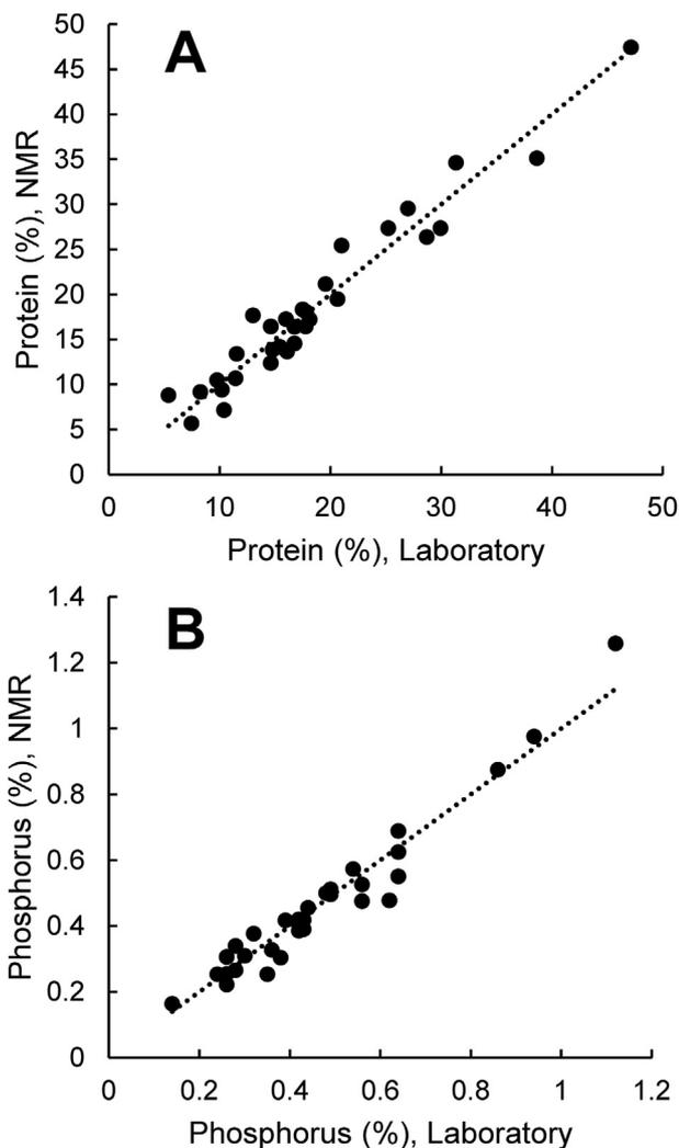
**Fig. 3** – Results of NMR measurements versus results from laboratory analysis for 31 feed samples. A) Calibrated  $^{14}\text{N}$  NMR results of enzymatically digested samples versus mean of protein analysis (Kjeldahl total nitrogen times 6.25) at two laboratories, and B) calibrated  $^{31}\text{P}$  NMR results using native feed samples versus laboratory analysis of total phosphorus. See text and [supplementary material](#) for details on samples, laboratory analysis, and NMR experiments.
